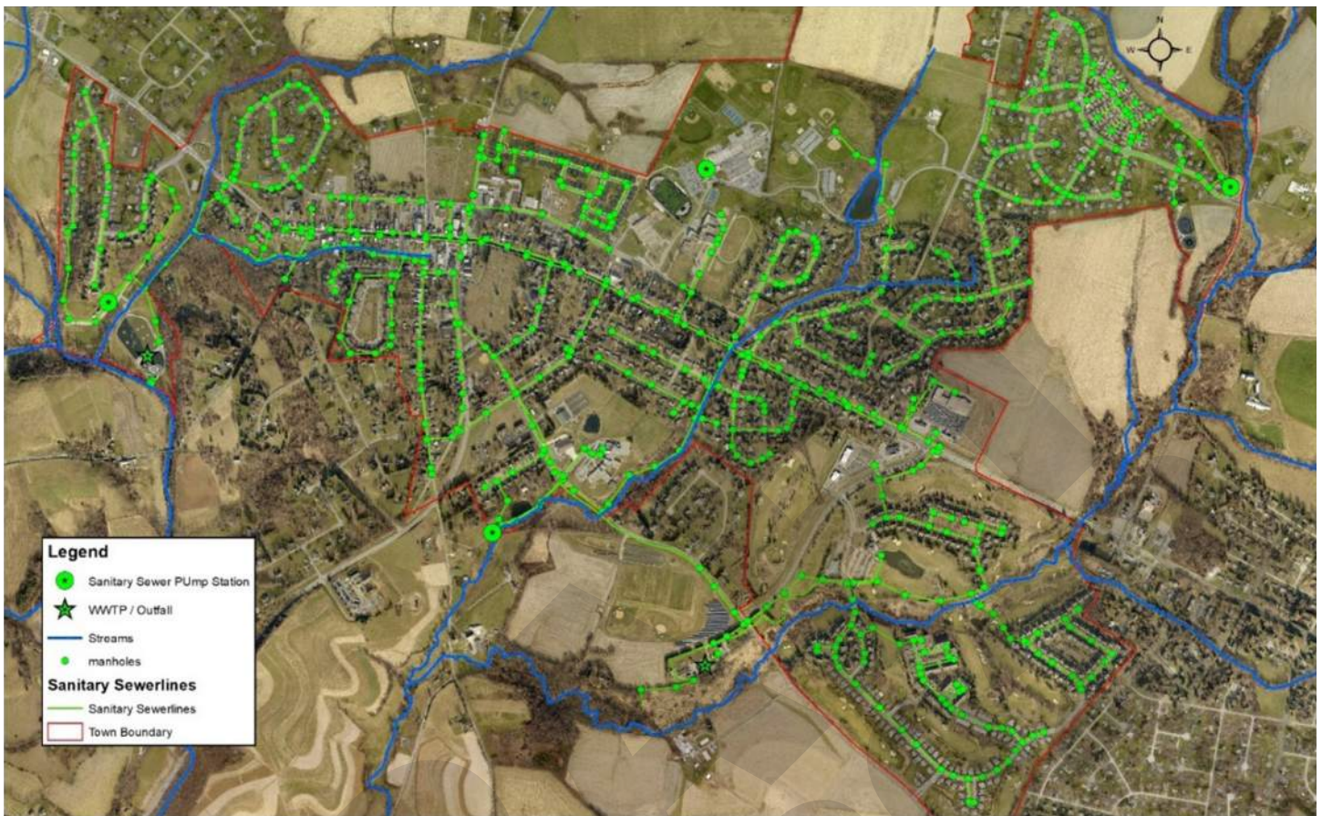
Figure 8-6 | Middletown Sanitary Sewer System Map
