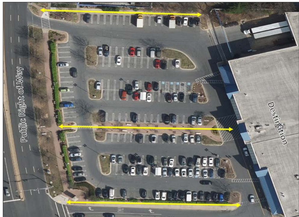
A shopping center on Hungerford Drive (MD 355) provides a direct pedestrian route from the public right-of-way through the parking lot and to the building entrance.
