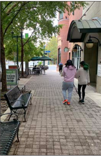
Pedestrians walk along Maryland Avenue in Town Center. There is ten feet of clear space for pedestrians to travel unencumbered by trees, street lights, benches, etc. Photo credit: City of Rockville.
